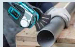
Cutting PVC, FRP pipes
