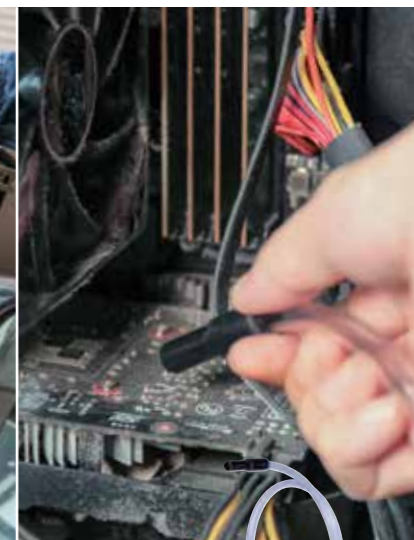
Flexible nozzle complete set Part No. 191X21-8 For blowing dust away from OA equipment or narrow spaces where this machine cannot enter
